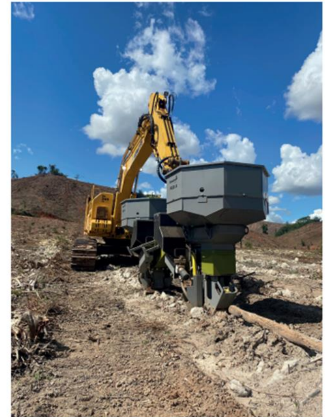
Bracke P22.b is mounted with a rotator and link that allows seedlings getting planted in a upright position
