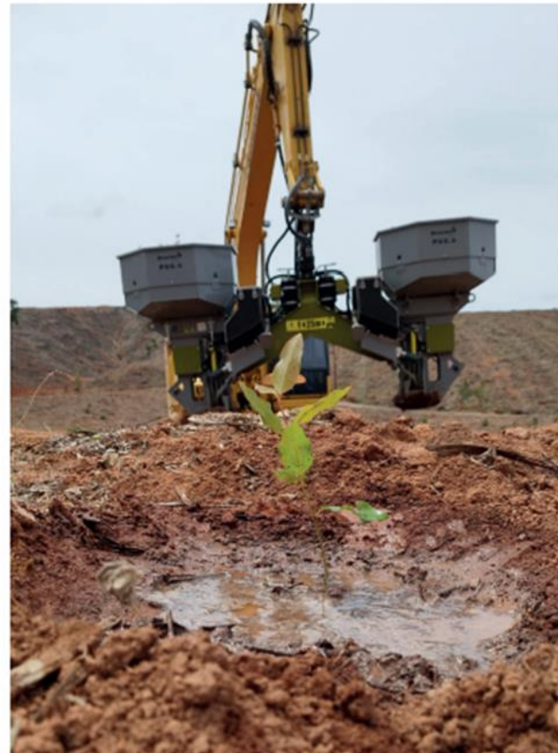
The Bracke P22.b has a low planting position to concentrate the irrigation water
